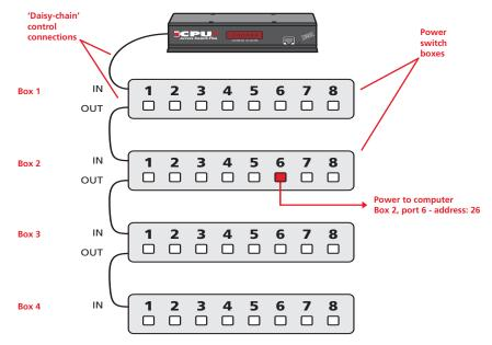
The power ports are connected to the power inputs of each computer and the power switch box(es) are then connected to a mains power supply.
